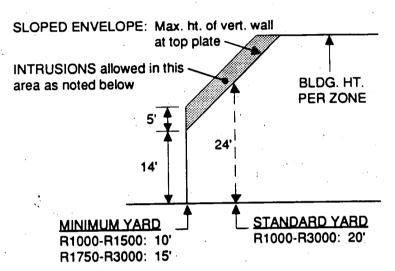
INTRUSIONS ALLOWED: Sloped roofs, dormers, open (60% minimum) balustrades, gable end vertical walls (chimneys and vents per code)
