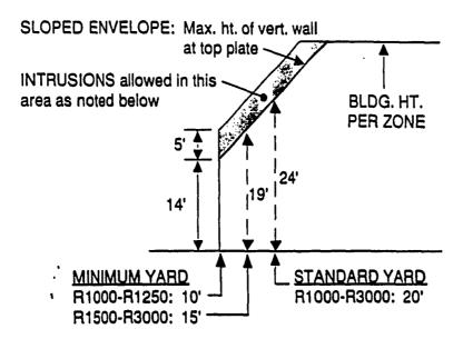
INTRUSIONS ALLOWED: Sloped roofs, dormers, open (60% minimum) balustrades, gable end vertical walls (chimneys and vents per code)
