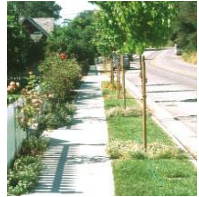
The photo shows non-contiguous sidewalk that is encouraged because it separates pedestrians from the vehicle
