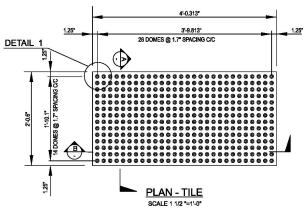
unique design that can be detected underfoot and with a cane. The research concluded that these other surfaces are not considered ADA equivalent and therefore, do not comply with the ADA requirements. Thus, truncated domes were determined to be the only acceptable detectable warning, under the ADA (See diagram above).
